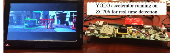
Figure 7: Accelerator for real-time car/pedestrian/cyclist detection generated by DNNBuilder
